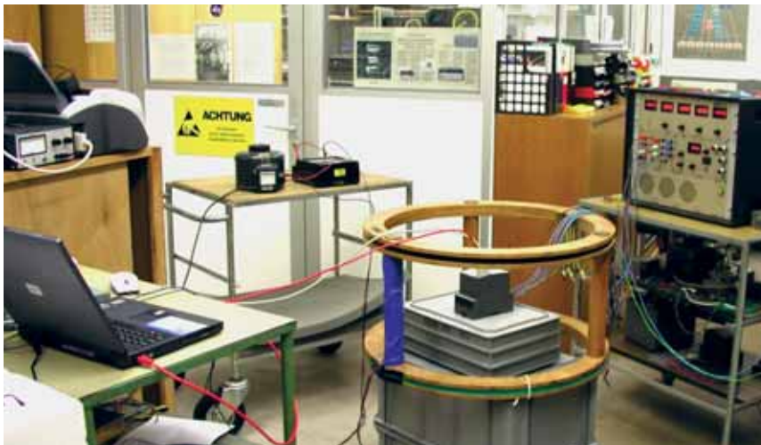
Determination of device behaviour under the influence of a magnetic external field generated by a Helmholtz coil
