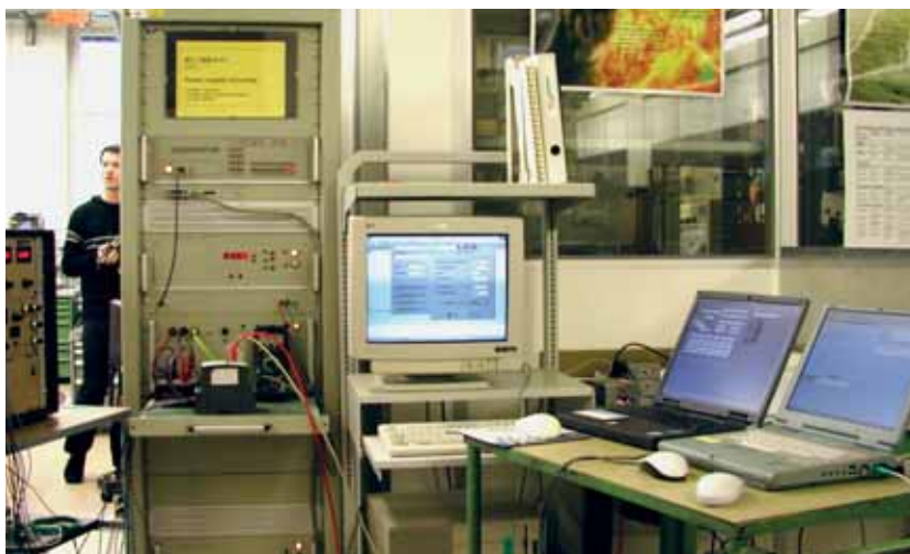
Measurement of the behaviour of the devices in voltage dips, brief interruptions or voltage fluctuations of the power supply
